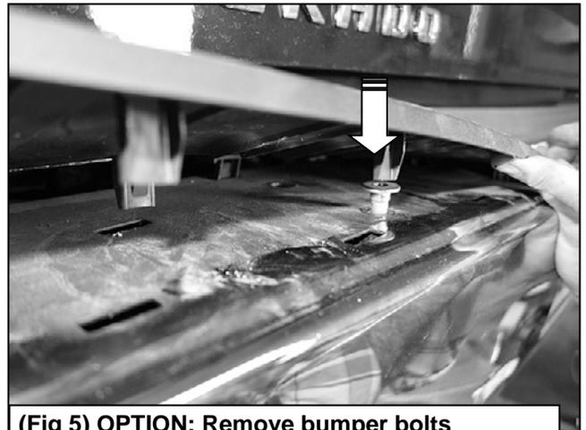
(Fig 5) OPTION: Remove bumper bolts attaching bumper to inner bracket. Remove outer bumper first, then remove inner brackets
