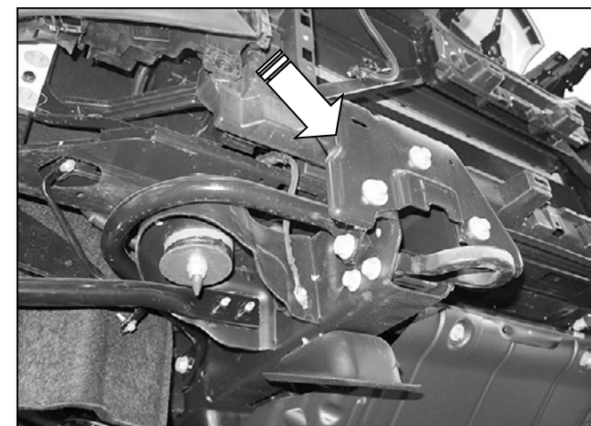
(Fig 6) Remove factory bumper brackets (Arrow)
