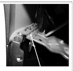
Fig6:Hold Top Bracket in place to determine area to cut from air deflector
