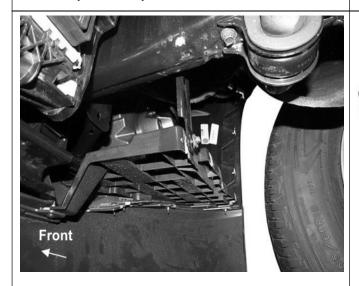
Fig4D:Pull back fender liner to access Bumper hardware and unplug light if equipped
