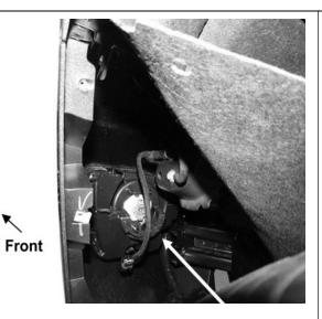
Fig5: Remove factory bolt (arrow).
