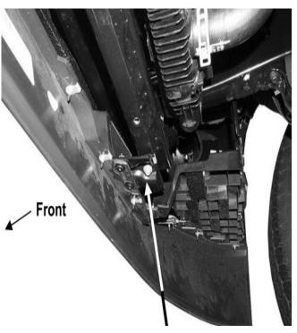
Fig4B: Remove hardware attaching plastic fill panel to inner fender
