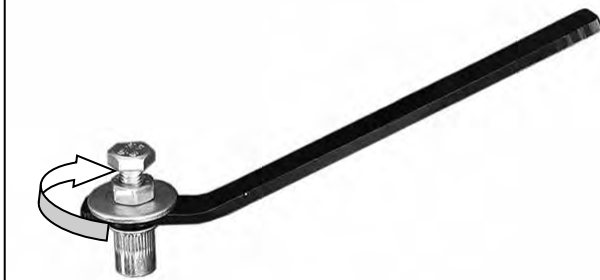
(Fig 5B) Assemble 6mm Insert Tool
