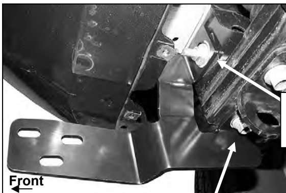
(Fig 5) Reuse factory hex bolt to attach Frame Bracket to bottom of cross-member
