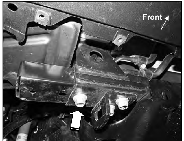
(Fig 2) Remove factory hex bolt (arrow)
