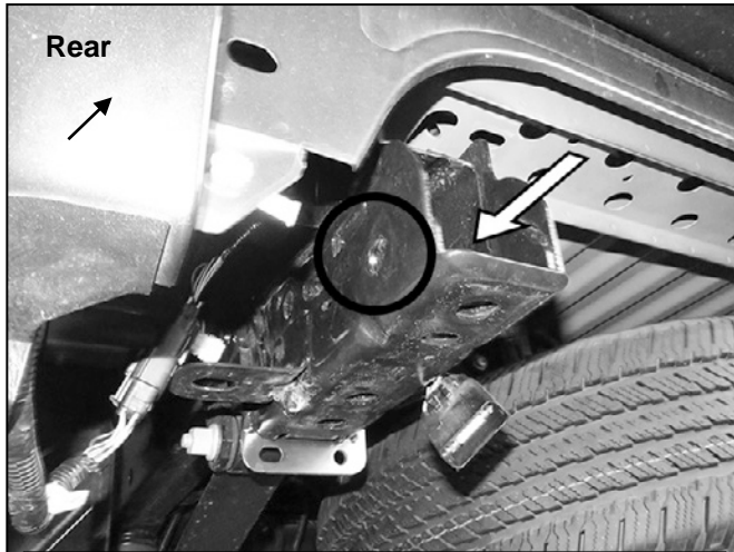
(Fig 5) Insert 10mm Single Bolt Plate into open end of frame and out hole in side of frame
