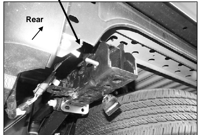
(Fig 6) Attach driver/left Frame Bracket to Bolt Plate
