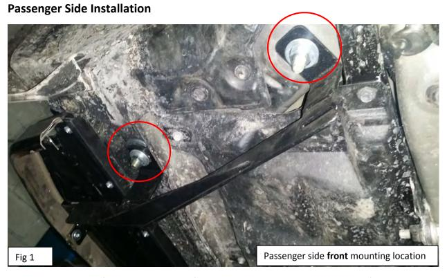
STEP2: Starting on the front passenger side of the vehicle, insert two drop pins into the factory holes. Select passenger side front mounting bracket and secure it with flat washers, lock washers and nuts. Do not tighten hardware at this time. (Fig1)
