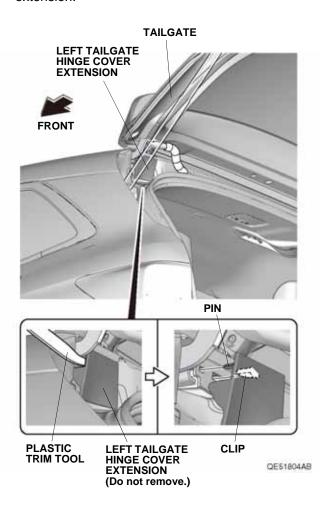
5. Close the tailgate halfway. Gently pry up on the rear edge of the left tailgate hinge cover, and remove it as shown. Do not reuse the left tailgate hinge cover.
