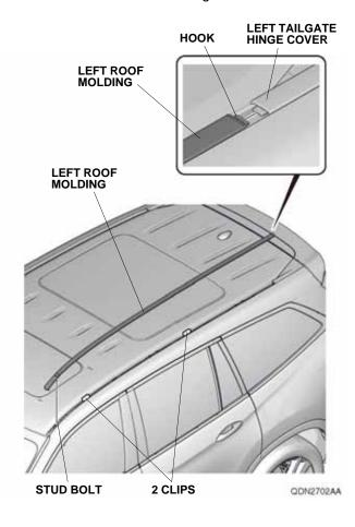
4. Open the tailgate. Using a plastic trim tool, release the left tailgate hinge cover extension as shown. NOTE: Do not remove the tailgate hinge cover extension.
