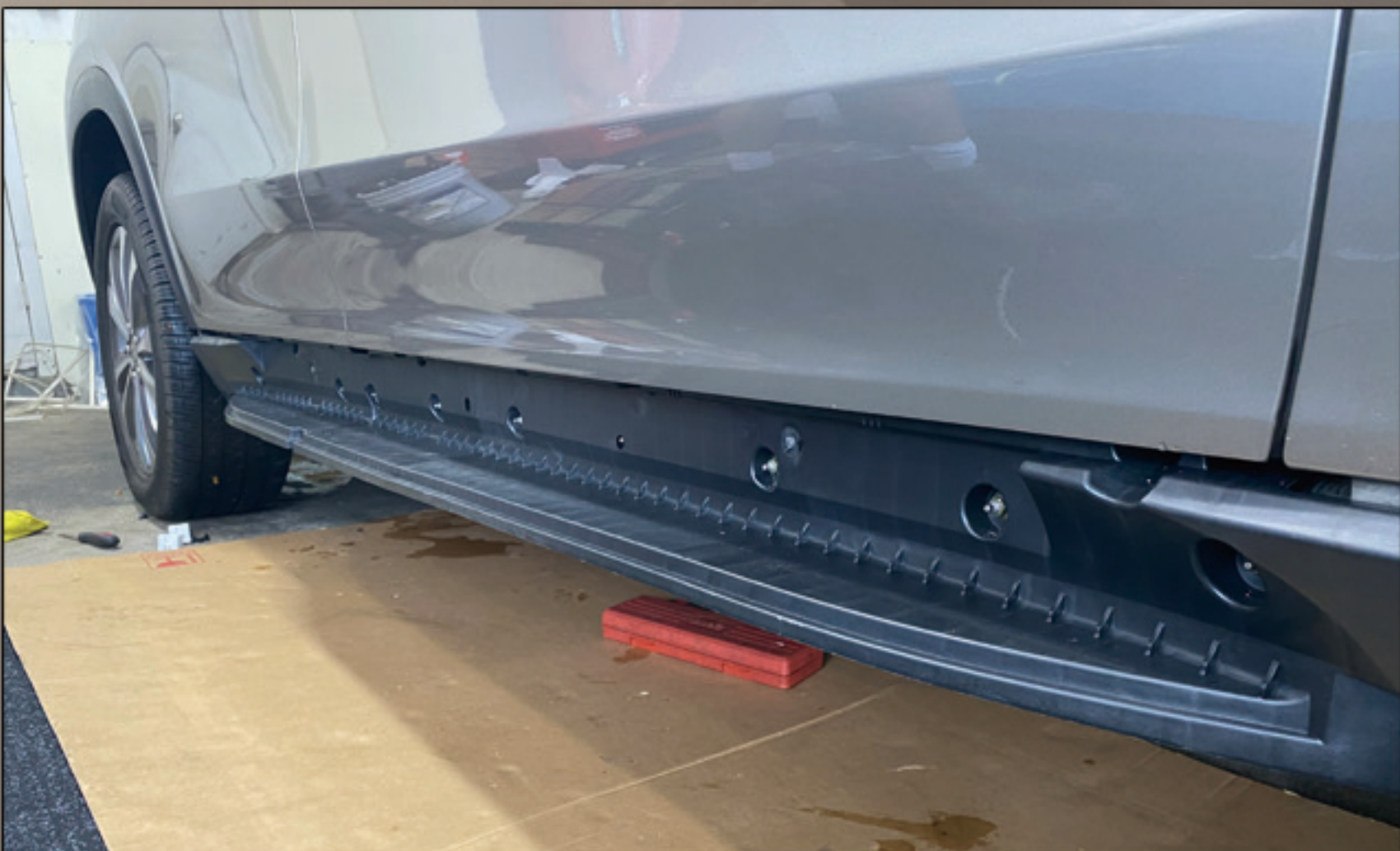
6.The internal bracket installation is complete.
