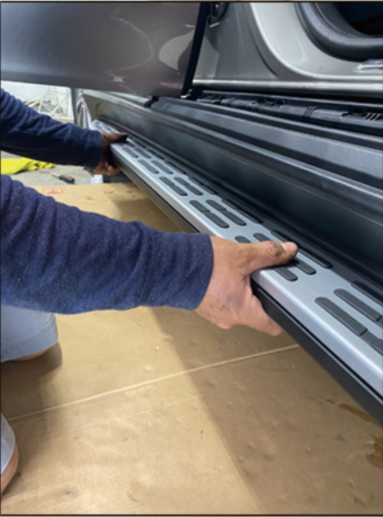
8.Install the outer pedal. Use air gun to fix.
