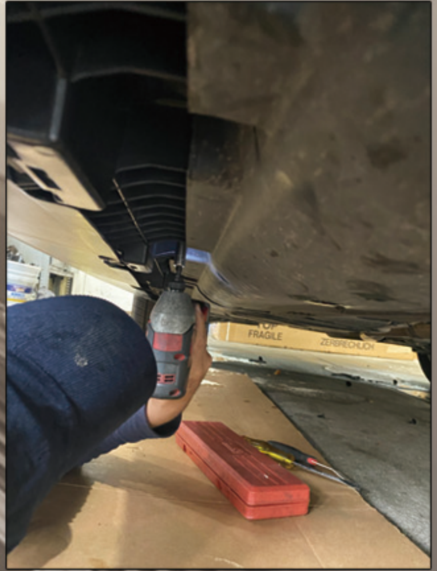
8.Install the outer pedal. Use air gun to fix.
