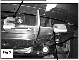
Slide Mounting Bracket between motor mount bushing
