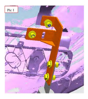
Step 3: Install the bull bar on the brackets and then adjust them to the proper positions.
