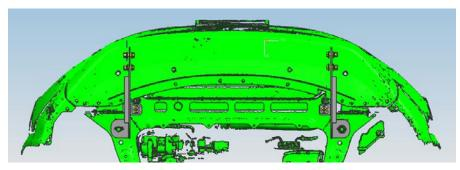
Step 3:Install the bar body on the bracket and adjust the mounting position of the bracket according to the position of the bar body.
