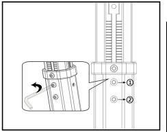
Loosen ①② screws properly, do not loosen all screws.
