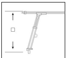
Loosen the screw on the post, adjust to the desired height, and observe the position of the scale value.
